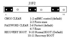
Figure 6. System Recovery and Update Jumpers (J1F2)
